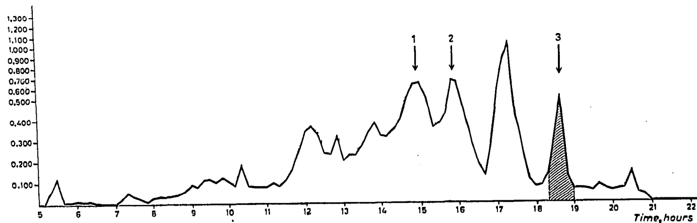
Fig. 3. Elution pattern of Hb N tryptic peptides from a Sephadex G-25 0.9 \times 120 cm column ( 0.2 N acetic acid; flow rate 60 ml/h). Arrow No. 1 = \beta\text{ATpIV} ; arrow No. 2 = \beta\text{ATpII} ; arrow No. 3 = \alpha^N\text{TpIII} .
